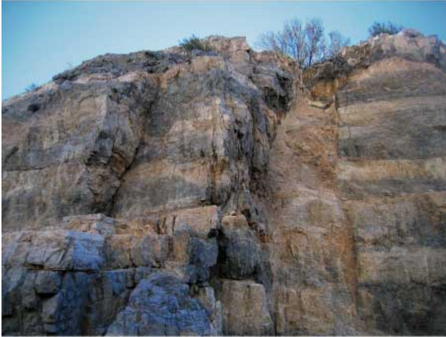
Figure 13. Fractures are most prevalent on the perpendicular faces, whereas those facing parallel are less broken up.
