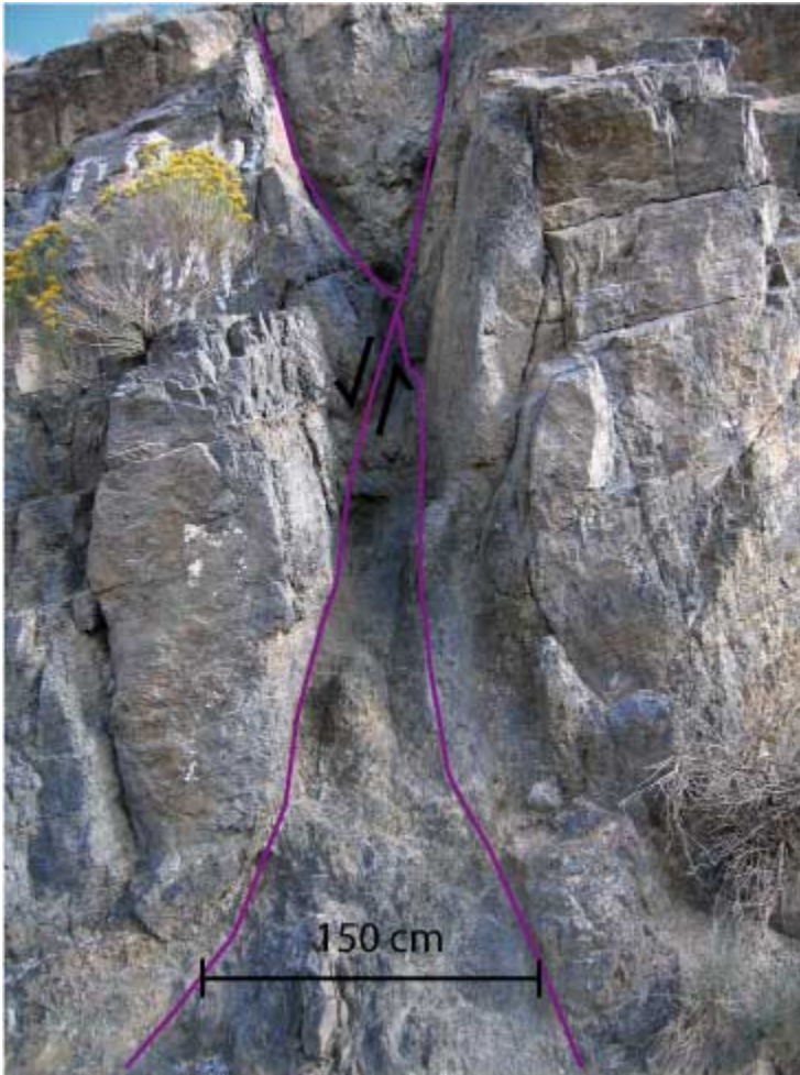
Figure 11. Localized shear along conjugate fracture set in limestone footwall. The blocks between fractures are broken into gouge in many places. The gouge zone here is about 150cm across at the bottom and decreases to 30cm near the top.
