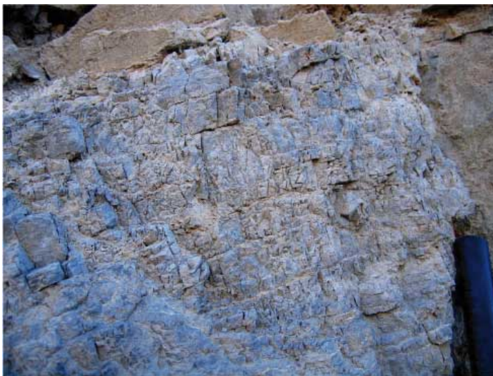
Figure 10. Intensely fractured limestone adjacent to core zone.
